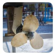
A three blade Max-Prop SailDrive equipped with Velox Plus being hauled out after a year at sea.
