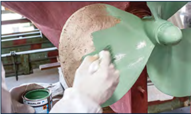
Applying Metal Primer.
