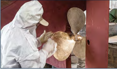
Wash and degrease all metallic surfaces with pure acetone.
