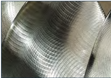
A Max-Prop propeller sanded thoroughly using 80 grit sand paper.
