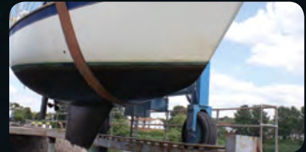
AFTER - Boat hull after being in the water for 2 years with the Sonihull system.
