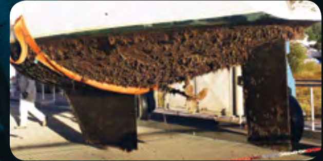
BEFORE - Fouling on hull prior to being cleaned, and then having Sonihull installed.
