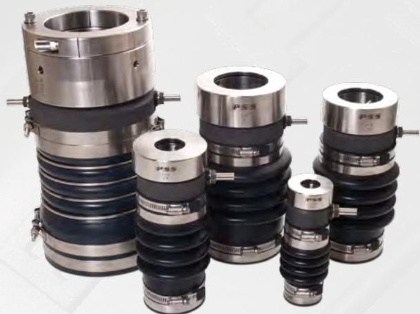
The Packless Sealing System (PSS) Shaft Seal is a mechanical face seal that is created between a rotating stainless steel rotor and a stationary carbon stator. The carbon stator is attached to a convoluted rubber bellow and the back of the bellow is attached to the shaft log (stern-tube) of the boat with hose clamps.
