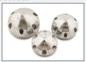
Keeping a quality sacrificial anode on your Max-Prop is critical to a long life for the propeller. Galvanic corrosion can destroy any piece of metal on a boat. A quality anode will help to protect your investment. PYI provides both Zinc and Aluminum anodes. All of our zincs have a metal ring molded into the anode to assist in disbursing the electrical current throughout the entire anode, improving the life of the anode.
