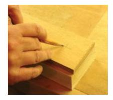
masking tape down and make a mark on that. Don't put it too close to the edge of the sole panel, and make sure it is closer than  $\frac{1}{2}$ " from the edge of the underlying support structure.
