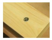
Use a small flat head screwdriver to fix the two parts together. The end result should be very neat and rattle free. If you would like go ahead and strategically place a little piece of hatch tape under the board to prevent any squeaks.
