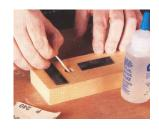
Spread a little epoxyon the countersunk ridges on the top anchor section.
