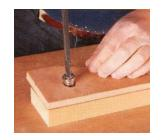
Screw the anchor down until countersink is flush with the surface of the floor panel, as shown. Wipe up any epoxy that squeezes out, and allow it to cure. The job is now complete.
