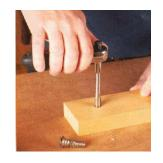
The next step is to open out the holes in the floor panel with the 13mm drill. A drill press is advised if you have the option. A handheld drill works fine, but make sure to keep the drill upright.
