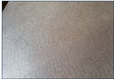
A propeller sandblasted.
