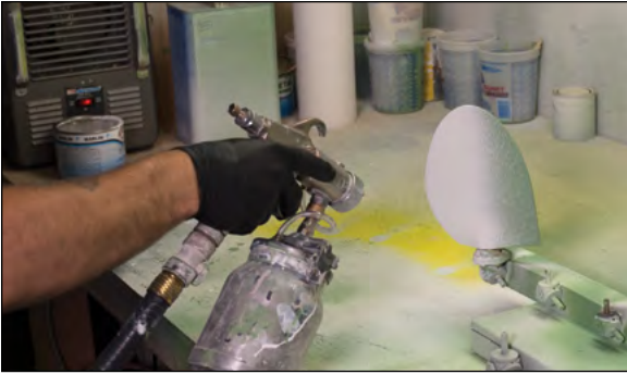
Applying first coat of Velox Plus Paint.
