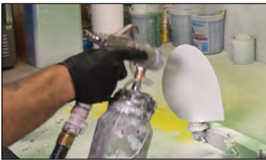
Applying second coat of Velox Plus Paint.
