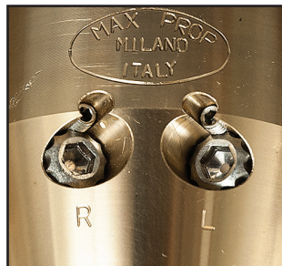
Fig.4 - Close up of the Left and Right pitch adjustment bolts.
